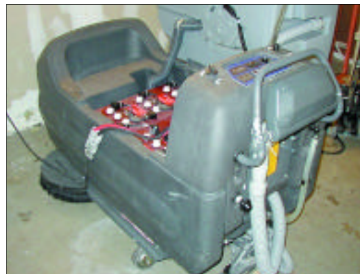
(Top) One of the industrial scrubber/dryers used by Xencom. (Middle) 36-Volt PowerPulse installed on the set of six 6-volt scrubber batteries. (Bottom) Using PowerPulse, run time on this floor burnisher went from three hours to over eight hours.
